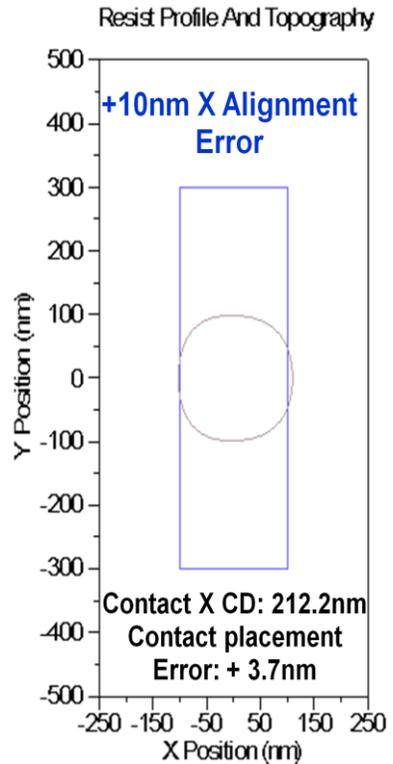
Fig. 8a. Slot exposure with +10nm alignment offset.
