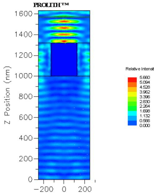
Figure 5. Prolith X3 simulation cross-section with a central line having gaps on each side.
