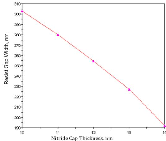
Figure 7b. Resist gap width versus nitride cap thickness.
