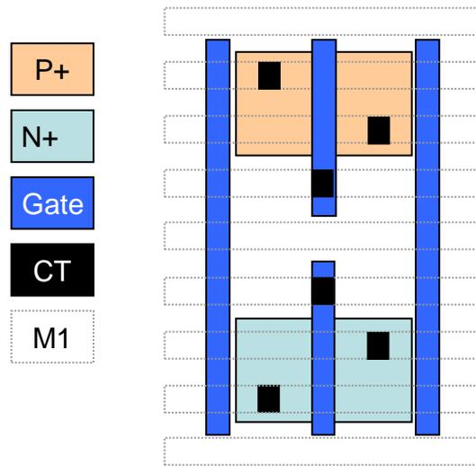
Figure 2. Logic inverter layout showing transistor layers.
