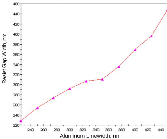
Figure 7a. Resist gap width versus mask width.
