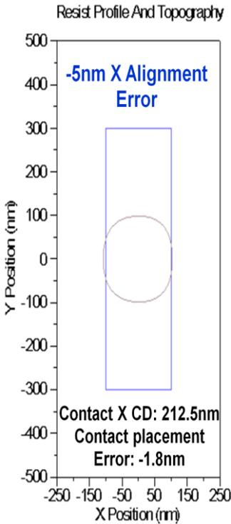
Fig. 8a. Slot exposure with -5nm alignment offset.
