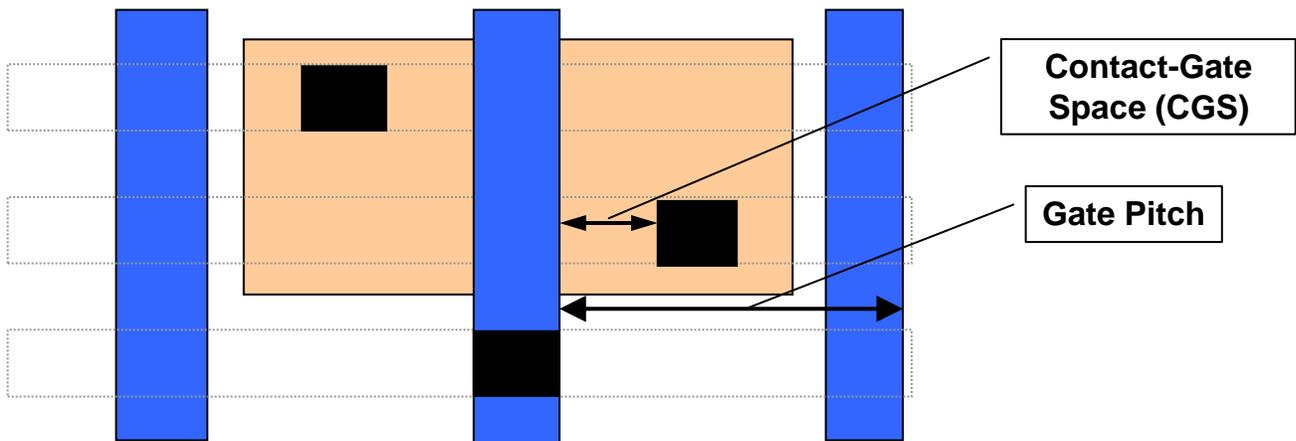
Figure 3. Detail of contacted-gate pitch.
