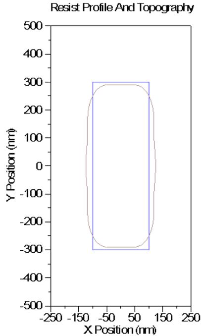
Figure 6. Aerial image (light brown) resulting from the original gate pattern (blue rectangle).
