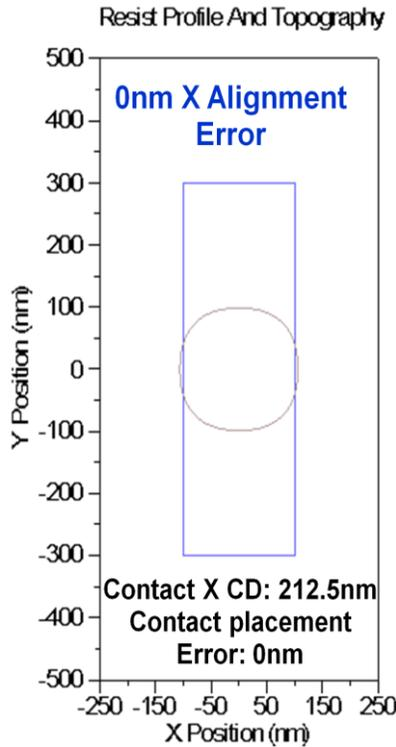
Fig. 8b. Slot exposure with 0nm alignment offset.
