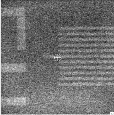
Figure 9a. Top-down SEM of the top resist pattern.
