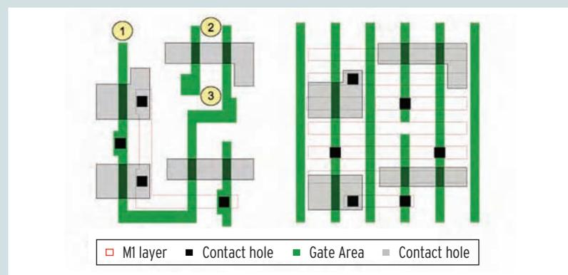
Figure S-1. (Left) 2-D complex design rule layout and (right) 1-D gridded design rule layout.
