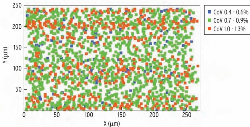
**Figure 4.** Gate CD uniformity for a logic block generated using aerial image simulation.
