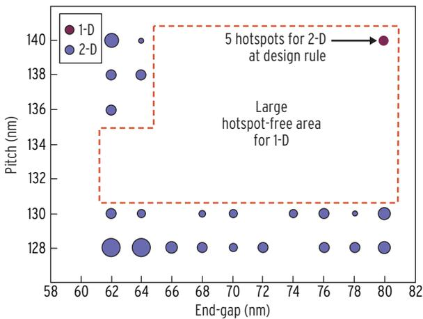
**Figure 5.** Metal-1 bridging hotspots. The diameter of the data point indicates the number of hotspots detected.
