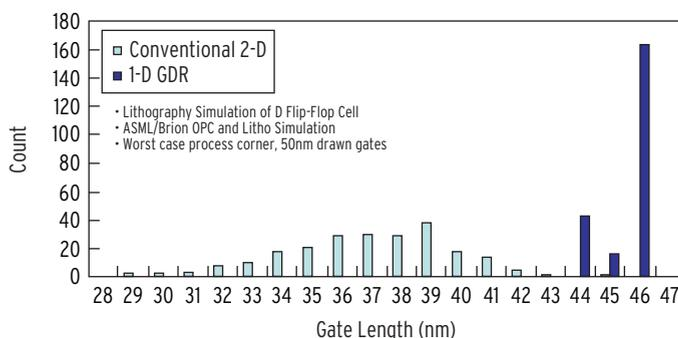
Figure 3. Gate CD distribution for 1-D and 2-D layout styles under worst-case simulated exposure process.
